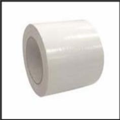
Geovex Seal Tape is a single-sided white woven tape that contains an acrylic adhesive with a release liner. It has excellent adhesion to polyethylene and the acrylic adhesive provides much longer life than many competitive tapes. It is recommended for taping the seams on in-wall vapor retarders and crawl spaces.
