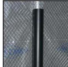
These full size clips are 11" long and fit most commercial scaffolding. Geo-Clips will securely fasten your poly sheeting to scaffolding, reducing wind whip and increasing the life of your enclosure. Clips are normally placed about every 3' onto the enclosure.
