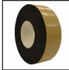
Butyl seal is a double-sided reinforced aggressive black butyl rubber tape used to join panels of polyethylene and polypropylene together by overlapping the edges and applying Butyl Seal in between. It is also used to adhere to concrete walls and footings when properly prepared. Butyl Seal is non-hardening and flexible.
