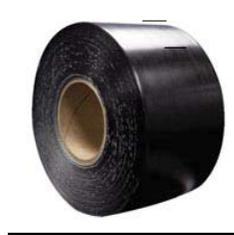
R25B Tape is a single sided aggressive synthetic elastomeric adhesive that bonds instantly to properly prepared polyethylene and polypropylene. The black polymer backing and adhesive is specially formulated to provide years of performance even in direct sunlight. A poly release liner provides for ease of installation.
