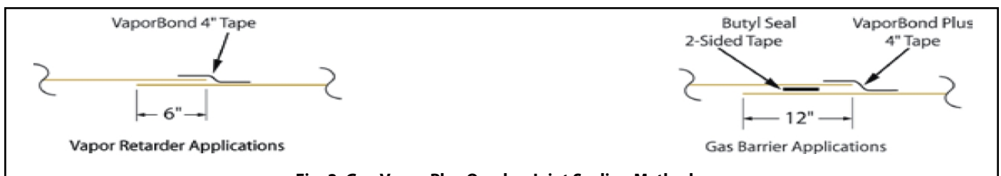
Fig. 2: Geo Vapor Plus Overlap Joint Sealing Methods
